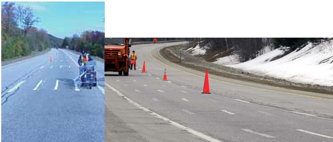
Traffic paint at the Lincoln test site. Left on October 9th 2002. Right on March 20 th , 2003.
