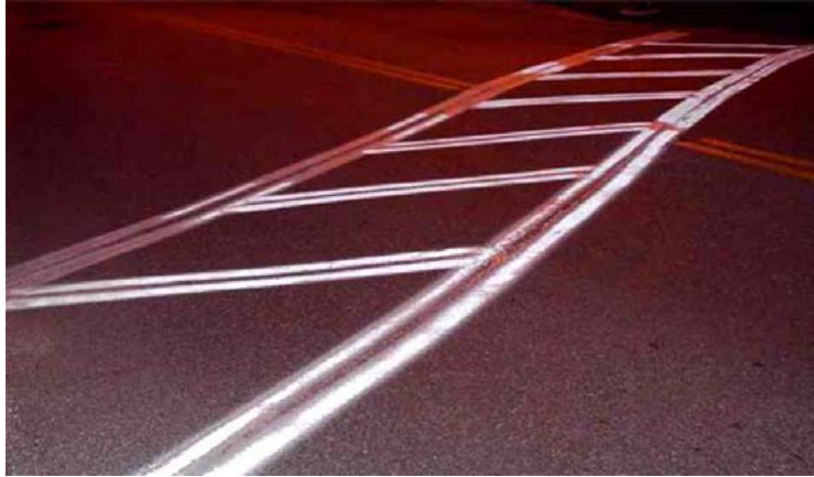
Figure 6: UNH test site after bead application
