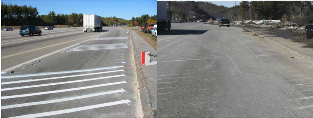
Traffic paint at the Hookset test site. Left on October 29th 2002. Right on March 16 th , 2003.
