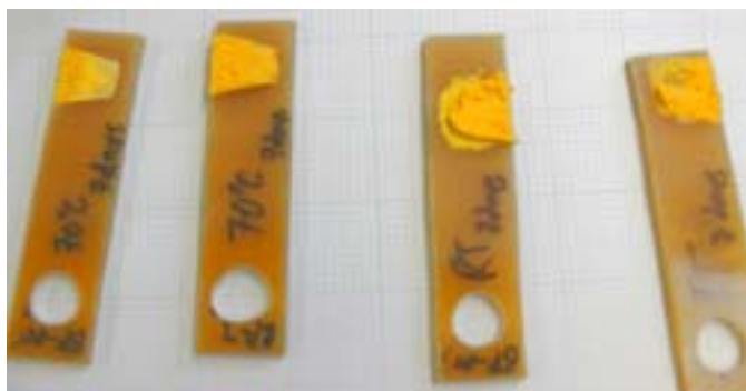
Figure 15: Samples made for initial Instron Test
