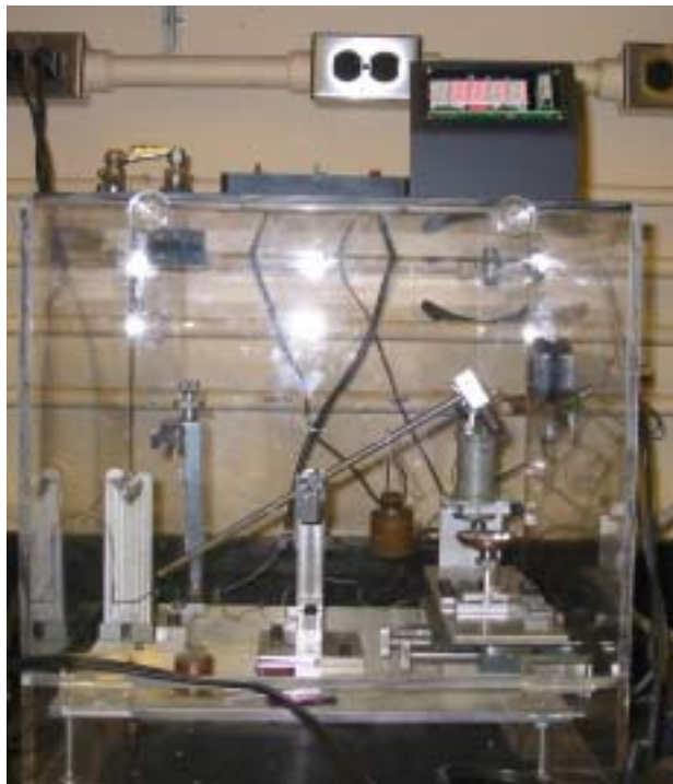
Figure 10: Wear Tester Developed at UNH Materials Science Department
