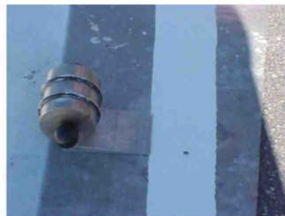
Figure13-d: ASTM D711 No-pick-Up wheel and ramp
